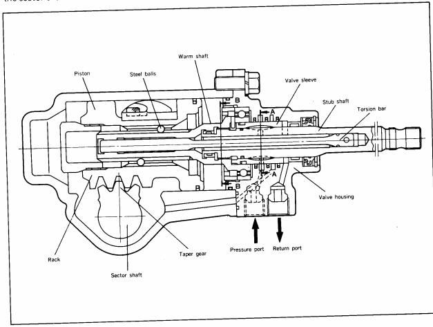
**For the power cylinder section** the inside of the steering gear box has been worked into a cylinder, and inside this there is a piston with the added function of a ball nut, thus making this a double-acting power cylinder.
