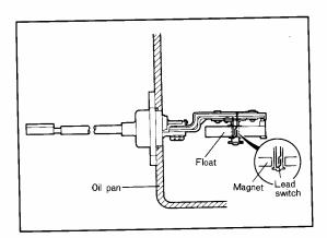
3. The float type has a magnet inside the lead switch, thus improving performance resulting from engine vibration.
