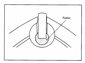
4. In order to prevent this, a rubber seal was added to the corner seal, as shown in the figure. This seal acted, without cramping the apex seal even if there was a slight manufacturing error of the groove width or the seal width, to maintain constant contact and to maintain airtightness. As a result, fluoric rubber, with outstanding resilience and excellent heat-resistance properties, is used.
