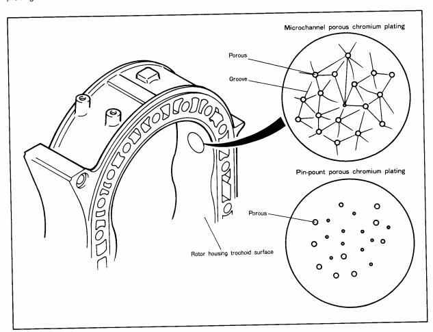
The objectives of microchannel porous chromium plating are to improve the oil retention of the rotor housing trochoid surface and to prevent chatter marks and vertical scratches caused by the apex seal. And, in addition, the plating hardness is increased by 20%, thus improving the durability of the rotor housing.
