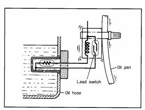
The lead switch of the thermistor type was clamped to the oil hose, with the result that engine vibrations were transmitted through the lead wiring to the lead switch, causing incorrect operation.
