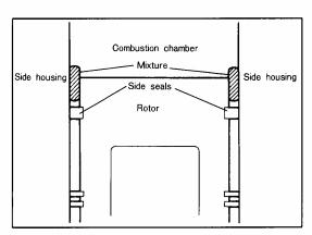
For the former rotor, the mixed gases (HC) in the shaded areas in the figure at the left were not completely burned, because of the low surrounding temperature, and were exhausted to the catalyst converter where they were oxidized.
