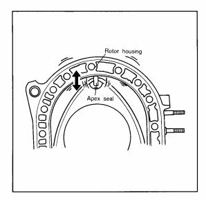
One of the primary causes of the chatter marks and vertical scratches, the sympathetic vibration (resonance) of the apex seal and rotor housing, was clarified by experiments.
