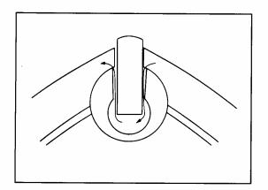
3. For that reason, it was necessary that the width of the groove of the apex seal used on the corner seal be greater than the groove in the rotor. But by doing so, a gap between the groove of the apex seal of the corner seal and the apex seal itself developed at both sides of the seal, and gases could easily escape from these gaps.
