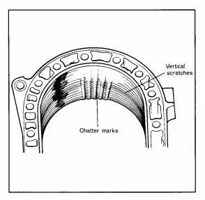
"Chatter marks" are the wavy, stepped wear which occurs on the rotor housing trochoid surface, and vertical scratches are, as their name indicates, scratches made by the apex seal in the rotor's direction of rotation.
