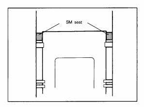
In order to even further improve the exhaust gas performance therefore, this SM (soft material) is coated, thus preventing mixture from reaching the zone where combustion is difficult, and thereby preventing the generation of incombusted gases.
