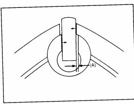
2. If the gap (A) between the apex seal and the corner seal is reduced to a certain value or less, the apex seal would be pressed on both the rotor groove and the corner seal, movement would be hindered, and the seal's performance would be reduced.
