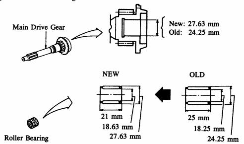
2. The method of retaining the bearing on the main shaft has been changed from clips to thrust washers with retaining rings.
