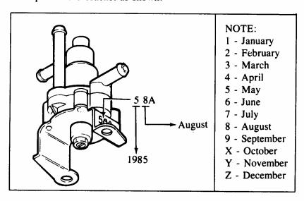
The check & cut valves produced on and after the following date are the modified ones.
