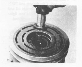
Insert the seal remover and installer tool against the seal assembly. Press down against the seal spring and twist the tool until feeling it engage in the slots of the seal cage. Lift out seal assembly.
