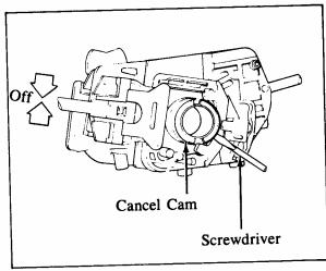
7. Align the tabs of the cancel cam with the holes in the steering wheel and install the steering wheel.
